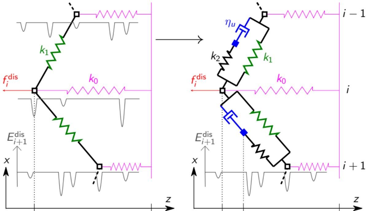
$$\eta \partial_t h_i = k_0(w - h_i) + f_i^{\text{dis}}(h_i) + k_1 \nabla^2 h_i + k_2 (\nabla^2 h_i - u_i)$$
